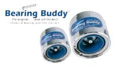
1980 Bearing Buddy w/Auto Check When the hub is full of grease the blue auto check ring rests about 1/8" outward from steel retaining ring. 1.980" Hub
